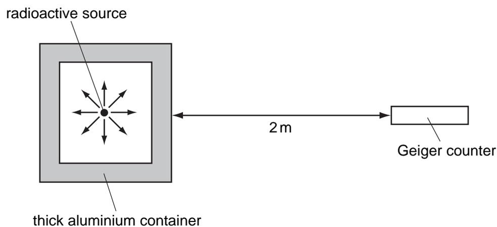
Which type of radiation from this source is being detected?
