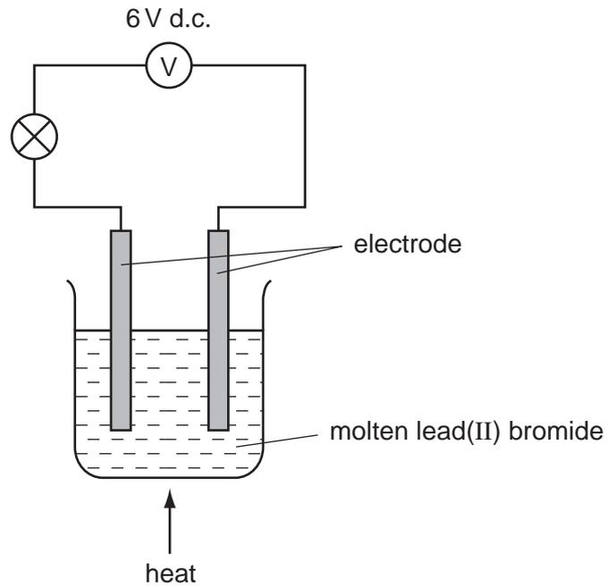
The bulb goes out soon after the heat is removed.
